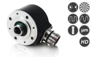
The encoder A58HM is used to measure angular position of the key machine components, industrial robots, comparators, rotary tables, servo drives and to establish an informational link with DCC, NC or Digital Readout Units. The encoder has integrated stator coupling so it can be fixed directly onto object shaft. Mounting adapter - similar to adapter of encoder A58H - is available on request.
