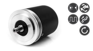
Absolute single turn rotary encoder AK50 is designed to be used in rotary tool changers, it features 8 bit gray or binary code outputs with arbitrary zero position, direction and resolution selection (set via switches), diagnostic facilities (status LED).
