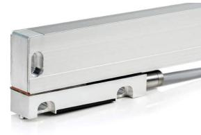
The sealed linear encoder L18 is used to convert linear displacements of key machine components into electrical signals containing information about the value and direction of the displacement.
