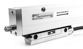
The sealed absolute photoelectric encoder LK24 is used to convert linear displacements of key machine components into electrical signals containing information about components absolute position.
