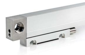
The sealed linear encoder L18T is used to convert linear displacements of key machine components into electrical signals containing information about the value and direction of the displacement. The difference from encoder L18 series is that it has the other housing fixation and more stable thermal behaviour.
