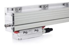
The precision sealed linear encoder L37 is used to convert linear displacements of key machine components into electrical signals containing information about the value and direction of the displacements.
